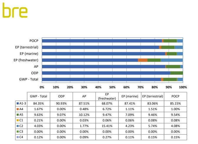
Figure 1 - shows the relative contribution of each life cycle stage to different environmental indicators for the carbon steel reinforcing bars manufactured by the Direct Reduced Iron production route
